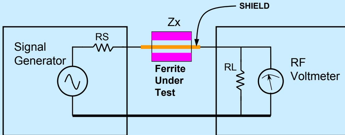
$R_S$  and  $R_L$  are generally 50 ohms
