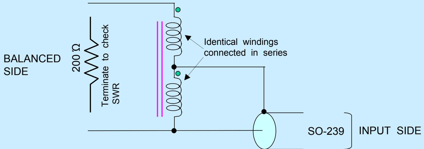
The measured inductance at the output is  $\sim 4X$  the input inductance as a result of inductance coupling.
