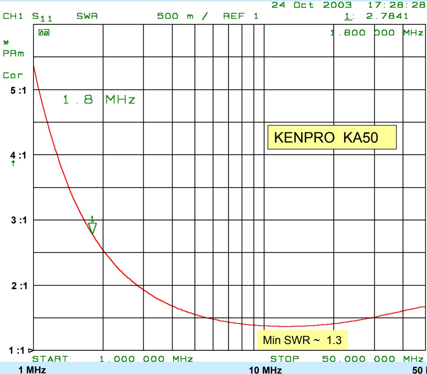
MEASURED SWR WITH A 200 ohms LOAD
