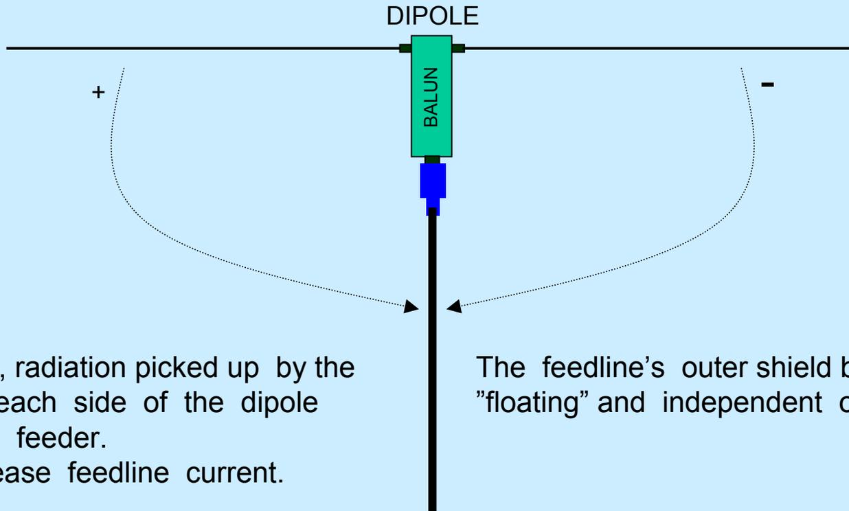
With a balun, radiation picked up by the feeder from each side of the dipole cancels at the feeder. This will decrease feedline current.
