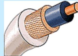
Note that the RF current that flows on the outer surface of the shield is independent of the inner shield current.
